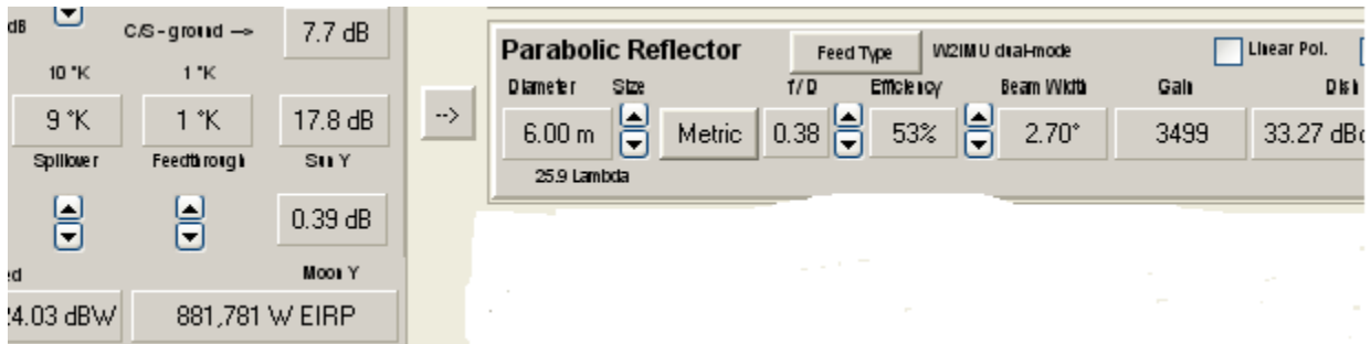
Figure 10 Antenna characteristics with W2IMU dual mode feed.
