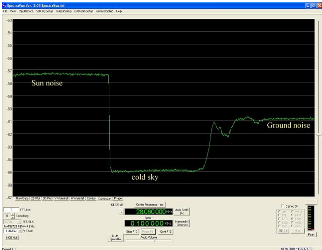
Figure 2 Spectravue SDR-IQ display of Total Signal Power
